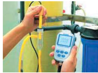
Conductivity/Resistivity Measurement of High Purity Water
